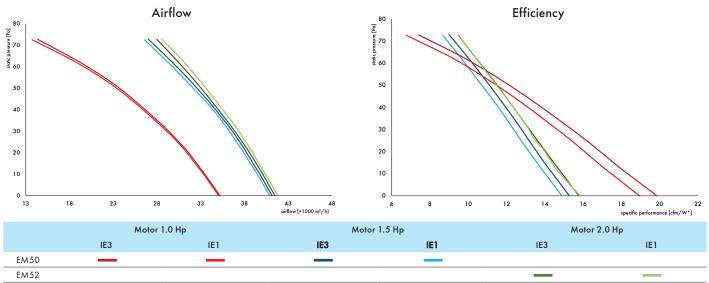
Airflow and efficiency data measured at standard conditions (20°; 1013 hPa). \*1 cfm/W =  $1.7 \text{ m}^3/\text{hW}$
